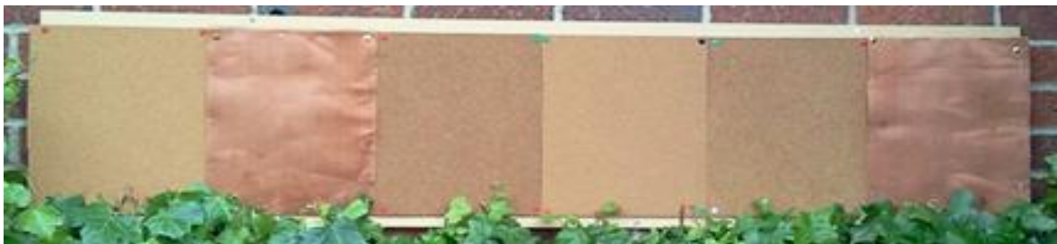
Figure 2 One of the model outdoor walls at the start of the outdoor experiment; it shows two replicates of the treatments (L to R: control, copper mesh, anti-graffiti paint 'Easy on', control, anti-graffiti paint 'Easy on' and copper mesh).
