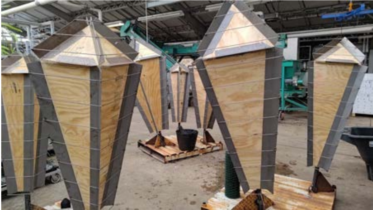
Custom made 'gem' forms made in-house by the metal shop
