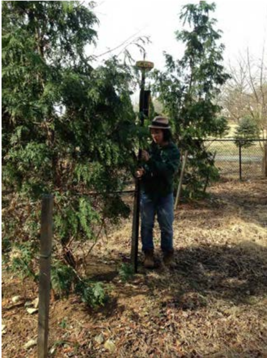
GPS mapping some Thuja occidentalis with a Topcon positioning system device,
