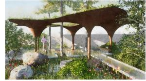
palustris and Hesperaloe parviflora. The pavilion is made of a steel subframe, clad with overlapping weathering steel sheets, giving it an organic and fluid form. Rainfall is harvested from the structure, filtering and slowing down its dispersal into the landscape.
